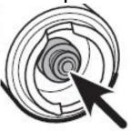
STEP THREE: Pull bulb out in direction of arrow below by pinching exposed portion of bulb with thumb and index finger (use or tweezers or similar tool)
